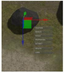
The Widget tool enable you to fine tune entities in your level, you can make tiny adjustments to the entities position, rotate around the x, y and z axis, scale the entities size, change its properties (more on that later), extract it completely, reposition it, delete it if you no longer need it or lock it in place so you don't accidently move it.
